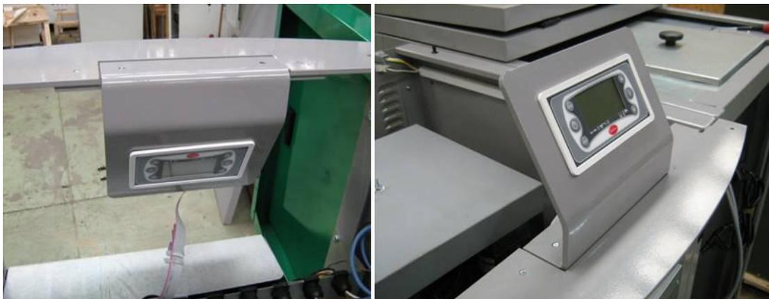
Re fit the control panel by screwing the screws from underneath the top support bar.
