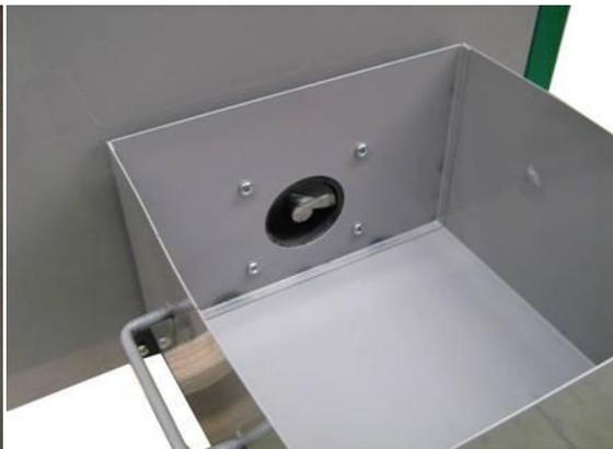
Slide the box onto the flange of the auger until it rests on the base. Cover the opening with the foil tape provided.
