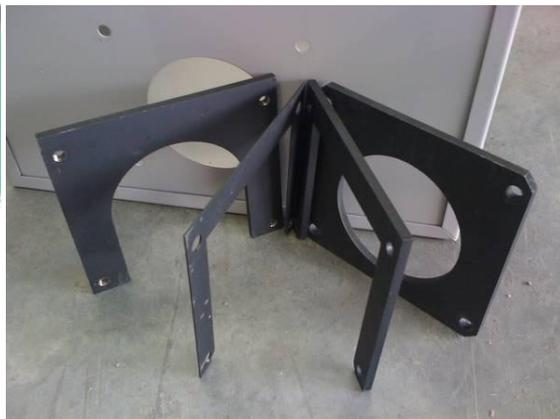
Fit the fixing plates for the de-ash box in the order shown above.
